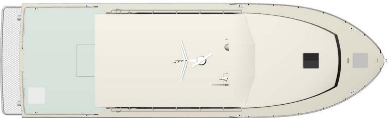
LOA: 14.0m Lmoulded: 13.2m LWL: 12.2m Beam: 4.00m Draft: 1.00m Fuel: 2500lts Water: 500lts
