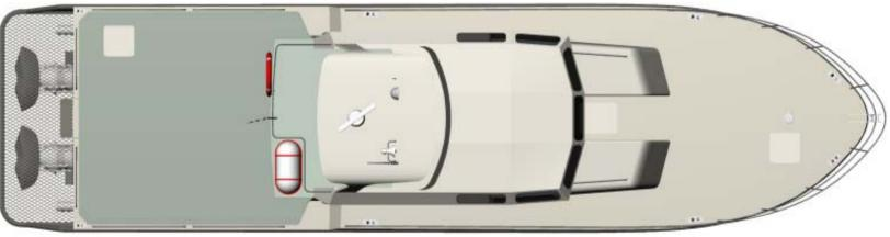
LOA: 17.5m Lmoulded: 16.1m LWL: 14.9m Beam: 4.60m Draft: 0.80m Fuel: 4000lts 2 x 882kW Power: Speed: 42 knots
