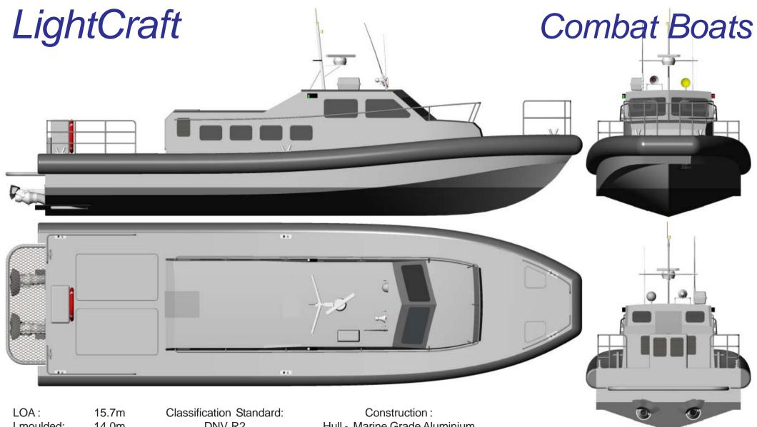
Lmoulded: 14.0m LWL: 13.3m Beam: 4.45m Bchine: 3.80m Draft: 0.6m Deadrise: 18deg. DNV R2
